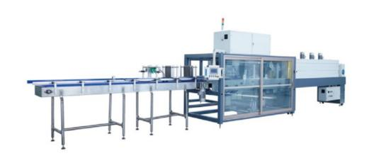
A complete packaging line includes not only bottling but also subsequent secondary packaging and end packaging. The secondary packaging is available in shrink film packaging, carton packaging, carton wrapping, etc. The end packaging can also be mechanical palletizing or robot palletizing.
