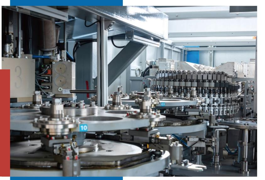
The blow molding machine first heats the PET preform, and then stretches and blows it with compressed air in the mold, in line with the development trend of high-speed beverage production lines, fully automatic rotary blow molding machines have gradually become the mainstream and are widely used by large and medium-sized beverage companies.
